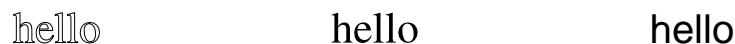
Figure 13: An illustration of the different ways that text can be imported: as letter outlines (left), as filled shapes (middle); or as characters (right).
