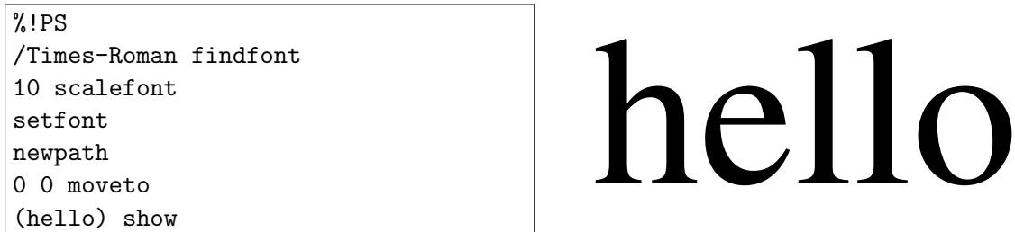
Figure 12: The file hello.ps , which contains PostScript code to draw the word “hello” in a Times Roman font. The resulting image is shown to the right of the PostScript code.
