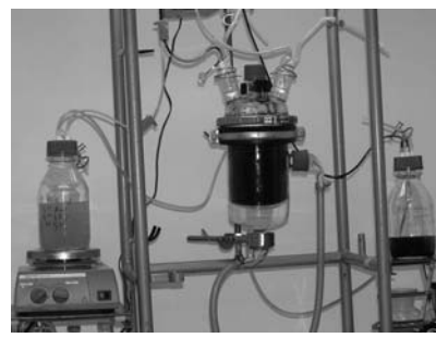
Fig. 3. Bioreactor during nutrient medium exchange.
