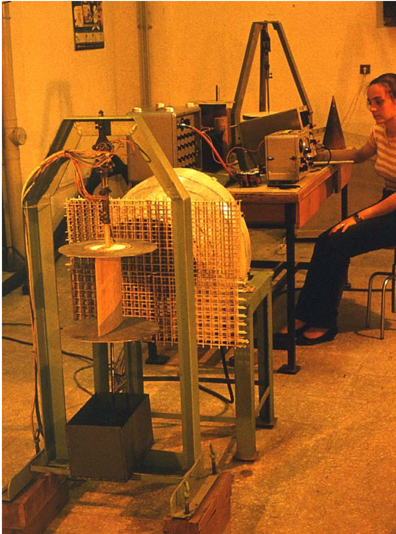
Fig. 3. View of the little free jet wind to determine the profile polar and the used measuring apparatus between the two limited discs.
