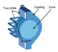
(a) Assembly of casting, core and chills(STL)
