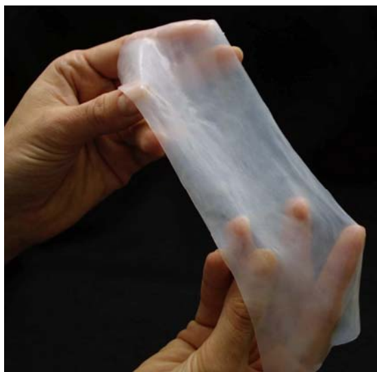
Fig. 1. Picture of original BC made by static fermentation (the source: fzmb GmbH)
