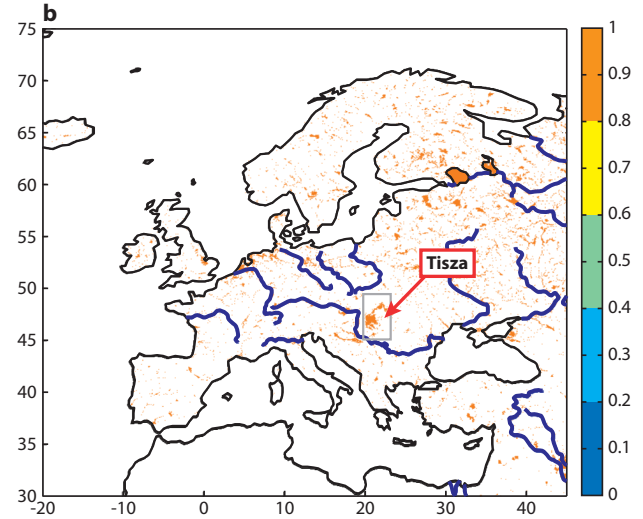
Fig. 5b. Flooding of 1 km by 1 km cells for a 50 yr return period focusing on Europe only (binary map). Major European rivers are shown as blue lines.
