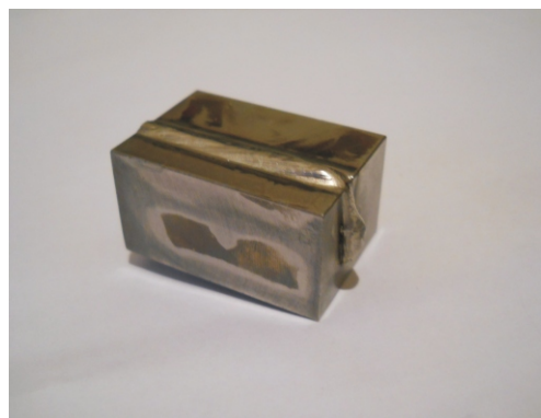
Figure 3(c). Bulk steel material welded by electron beam
