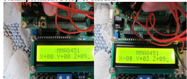
Fig.6 "accelerometer values at different head positions"
