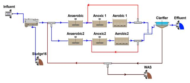
Figure 2 Biowin model of Moreni WWTP based on A2/O process
