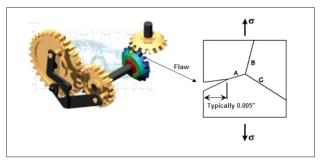
Figure 4: Initial flaw formed in the grain boundary
