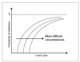
Figure 2: Crack Probability of Detection Curves.
