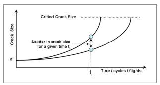
Figure 3: Scatter in Crack Growth Curve.
