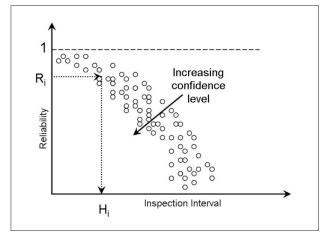
Figure 9: Overall reliability as function of Inspection Interval.
