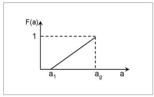
Figure 1: CDF for initial crack size.
