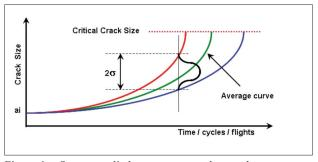
Figure 6: Scatter applied on average crack growth curve.
