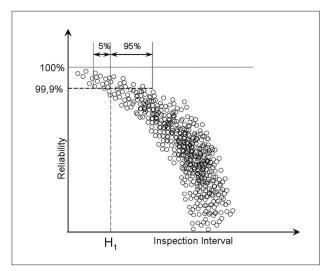
Figure 10: Inspection interval H<sub>1</sub>, given 99.9 per cent reliability, with 95 per cent confidence level.
