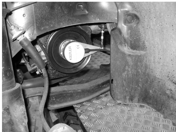
Fig. 3. Special container for gaseous fuel (A) and engine crank angle encoder (B)
