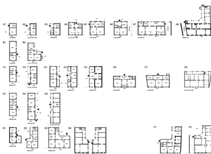
Figure 1. Ground floor plans of different type of ground floor houses in Subotica built in 19 th century showing transformation lines from simplest two room rural house to most developed types of urban ground floor houses
