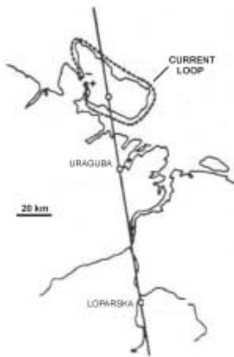
Fig. 14. Current loop arrangement and the profile for magnetic measurements of the “Khibiny-Experiments”, performed at the coast of the Barents Sea in the period 1976 to 1987 (Velikhov, 1989).
