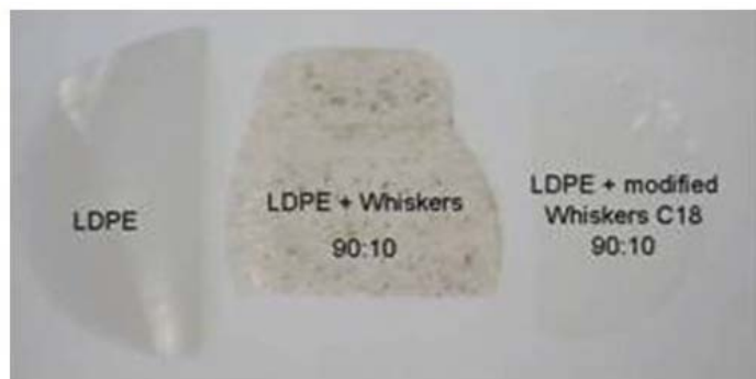
Figure 6. Photographs of the neat LDPE film and extruded nanocomposite films reinforced with 10 wt % of unmodified and C18 acid chloride-grafted cellulose whiskers [86].
