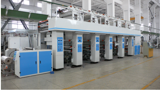
FIGURE 4: Experimental setup of the four-color gravure printing machines.
