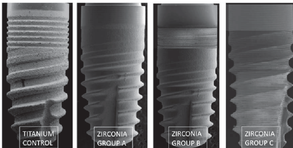
Fig. 2 – Scanning electron microscope (SEM) image composition of implants used in this study. The control implants have microthreads at neck level. All the implants have the same geometry. The laser processed surfaces of the group B and the group C showed the microgrooves at the neck level or in all surface, respectively.
