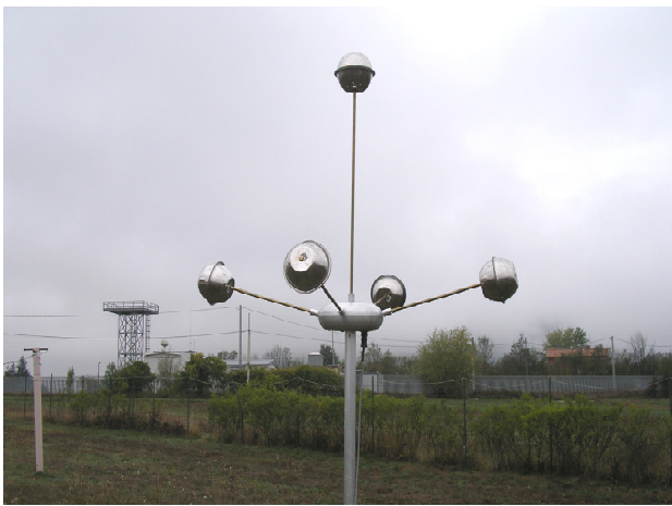
Fig. 2. Three axes antenna for electric field measurement in the frequency band [1 Hz–100 kHz]. The instrumental sensitivity 1 \mu\text{V}/(m\sqrt{\text{Hz}}) .
