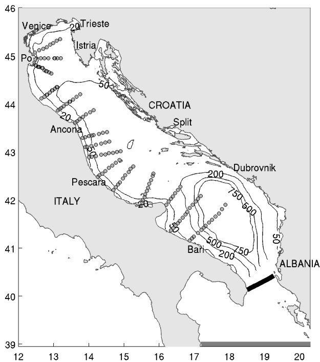
Fig. 1. Adriatic Sea coastline and bathymetry. Small circles represent CTDs locations. Note that iso-contours of depth 20 m, 50 m and 200 m, shown in the plot, are the very same used in the grouping done in Sect. 3. The grey thick line at 39°N represents AREG open boundary, while the black thick line at roughly 40°N represents AdriaROMS open boundary.
