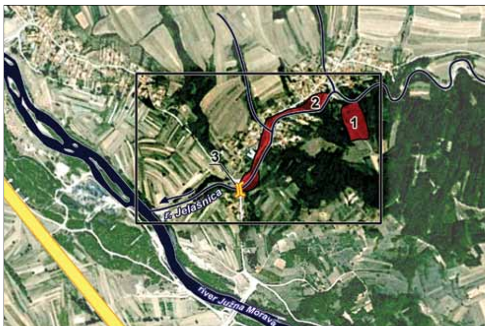
Figure 2. The Jelašnica river section through village Jelašnica (1 - landslide, 2 - flooded areas, 3 - the bridge)
