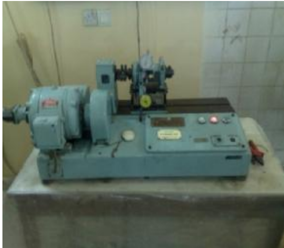
Fig. 2-6. a) AVERY Fatigue Testing Machine Type 7305, b) Close up of Specimen Fixture.
