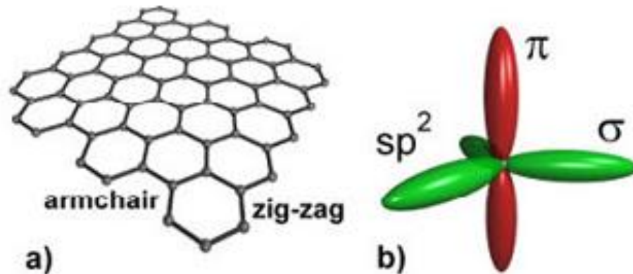
Figure 2.4: Armchair and zig-zag edges in graphene (a), sp^2 hybridization illustrated in graphene (b).
