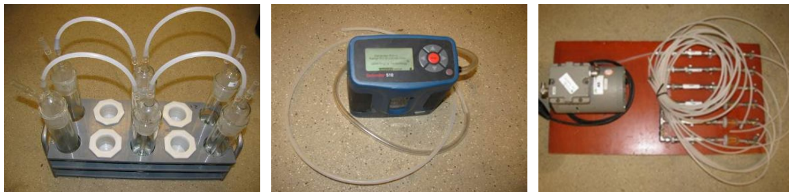
Figure 4.1 Set-up WLR gas washing method. Left: absorption flasks (measurements in duplicate; per train (in series) two absorption flasks filled with absorption medium and one empty absorption flask for protection of the pump). Middle: Dry gas flow meter (DryCal® Defender 510-m, Bios Int. Corp, USA). Right: pump (Thomas Industries Inc., model 617CD32, Wabasha, Minnesota ,VS), sampling lines (Teflon or polyethylene), and critical orifices (borosilicate glass (diameter: 8 mm; length: 80 mm), housed in a stainless steel container for protection; flow: ~1000 ml/min).
