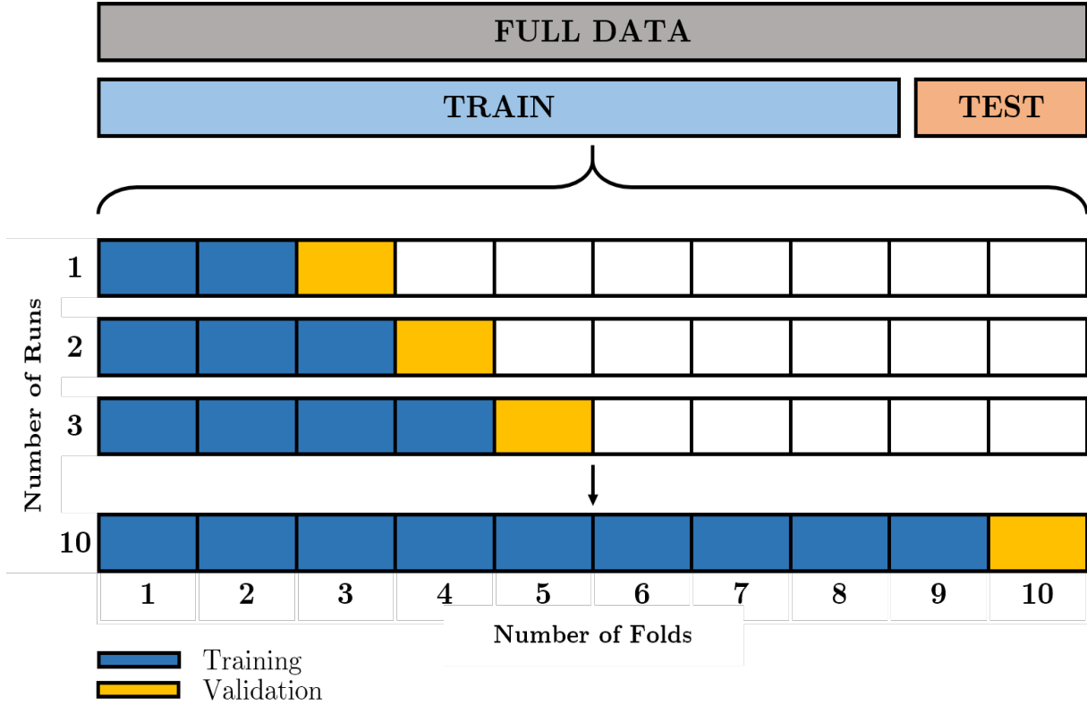
Figure 3.3: 10-fold cross validation process for time series data
