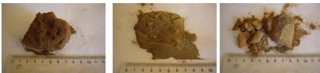
Figure 13. Ash deposits taken from superheater PP2A, fuel trials U100, U95B5 and U93B7
