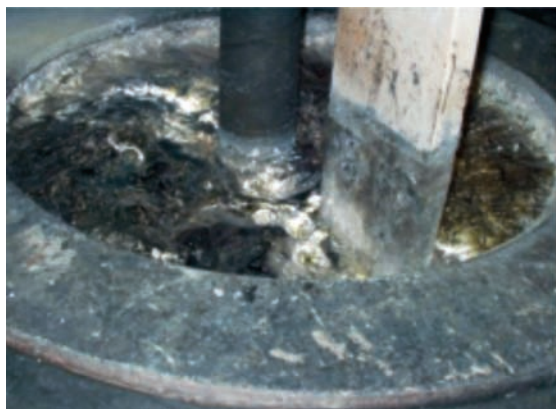
(c) Vortex removal, ~5 s, 350–500 rpm
