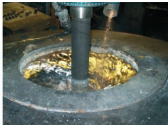
(b) Granular flux addition, ~30 s, 550–700 rpm
