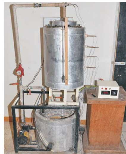
Figure 2. Photograph of TES tank with constant heat source
