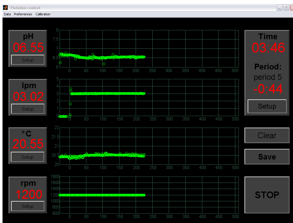
Fig. 4. Graphical user interface during a flotation test.
