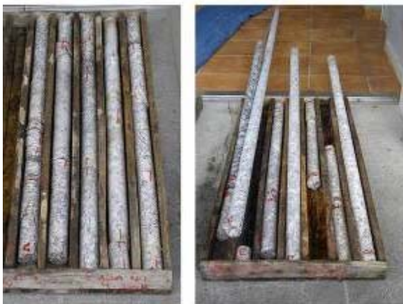
Fig. 9. View of the excellent granite drill cores recovered in the investigation stage.
