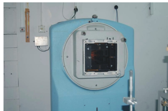
Figure 2. The ^{60}\text{Co} radiotherapy unit as source of gamma radiation for POF
