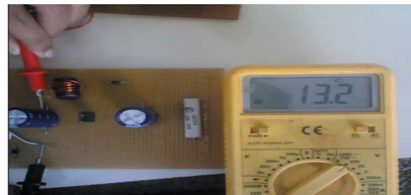
Fig. 4d. Display of the input voltage
