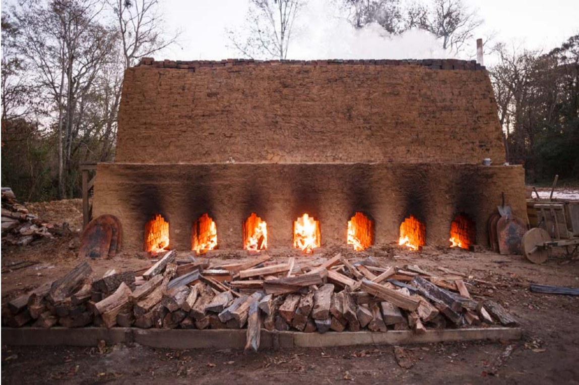
Figure 4.11: Clamp, Above Ground Example (“Trading Secrets: A Different Kind of Baking Project Bricks”).
