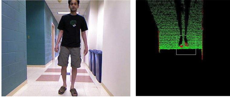
Figure 4.19: Generation of occupancy map from Kinect data
