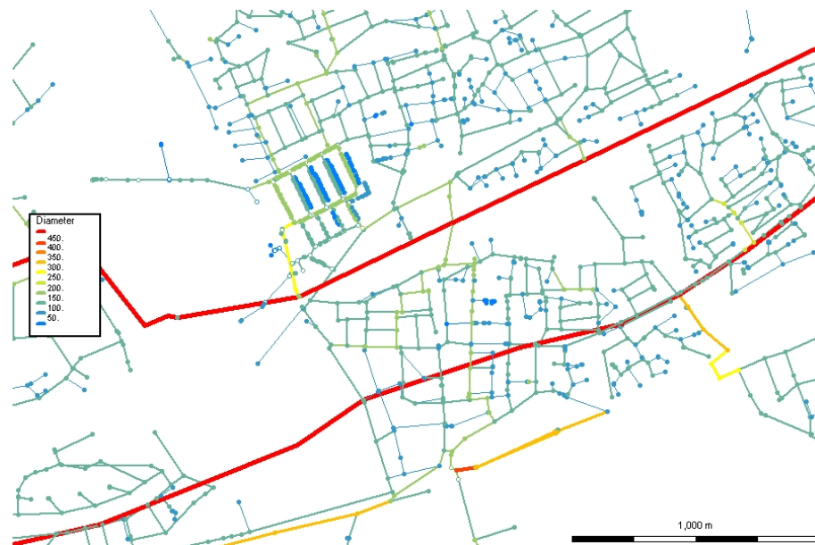
Figure 1. Part of a distribution network. The line colour and thickness represent the diameter of the pipes, the blue circles are demand nodes, open circles are nodes with zero demand. The thick yellow, orange and red lines are typically mains with a transport function (i.e. large diameters and very few demand nodes that are directly connected to it); the thin blue and green lines are mains with a distribution function (i.e. supply to customers).
