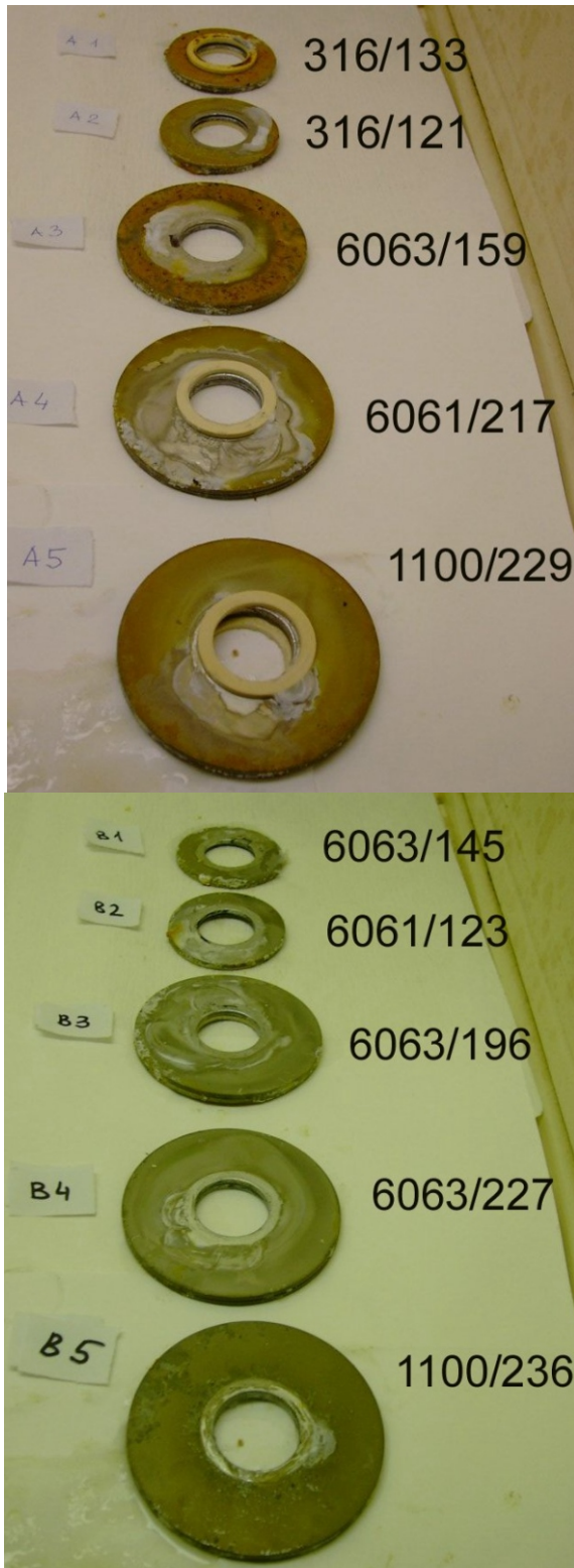
Figure 17. Front side (A) and backside (B) of coupons of disassembled Rack#2.1/CRP-I
