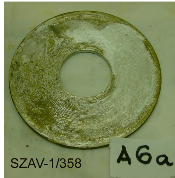
Figure 27. Crevice corrosion at the coupled side of coupon SAV-1/358
