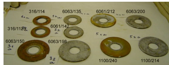
Figure 31. Front side (A) of coupons of disassembled Rack#2.2/CRP-I
