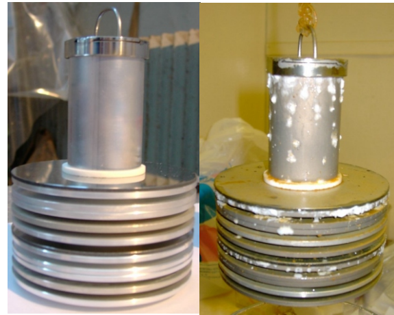
Figure 22. Rack#1/CRP-II before immersion and after 6 months of exposition time
