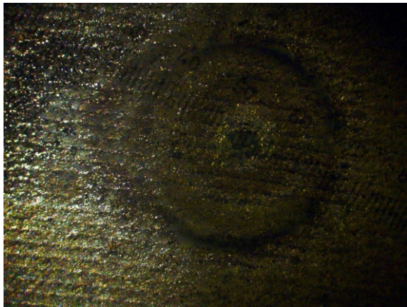
Figure 29. Circular pits at the top surface of coupon 6061/302 (magnification 10)
