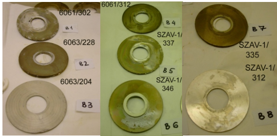
Figure 24. Back side (B) of coupons of disassembled Rack#1/CRP-II
