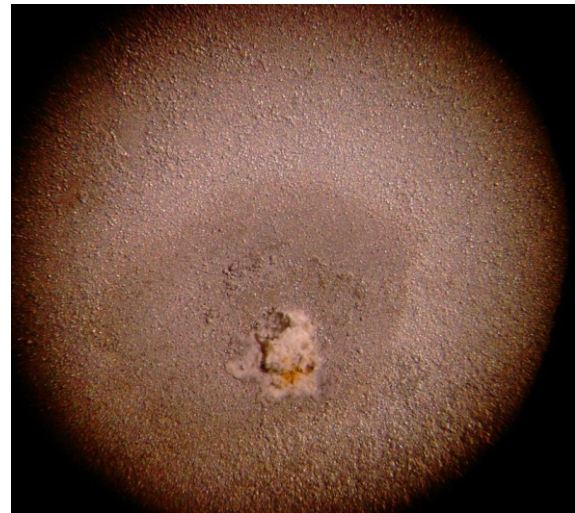
Figure 15. A pit covered with white blister at coupon SAV-1/60
