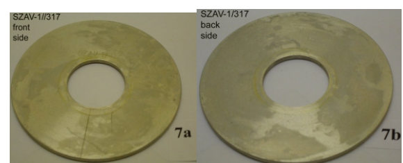
Figure 41. No corrosion observed at the single coupon SAV-1/317
