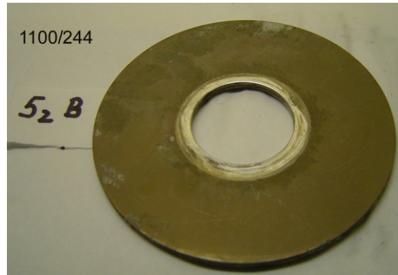
Figure 35. Uniformly dull surface of the front side of coupon 1100/244
