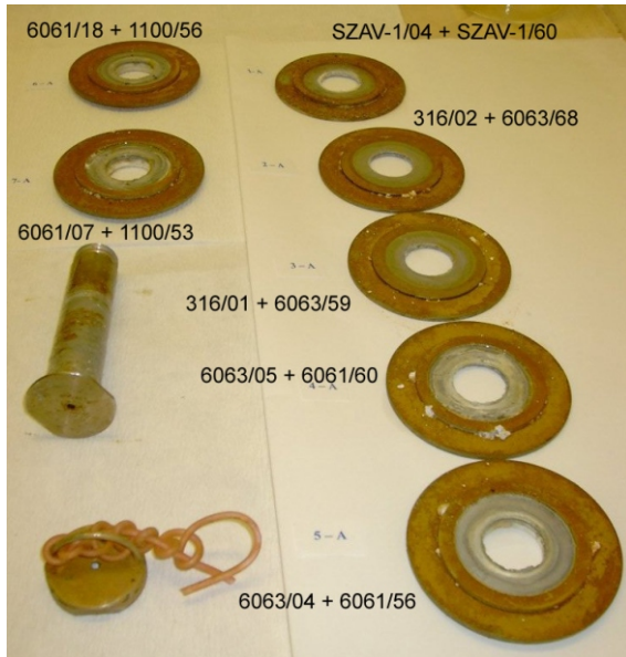
Figure 9. Front side (A) of coupon couples of disassembled Rack#1/CRP-I
