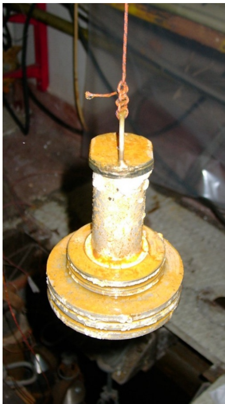
Figure 30. Rack#2.2/CRP-I after 24 months of exposition time
