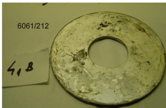
Figure 34. Crevice corrosion at the coupled side of coupon 6061/212
