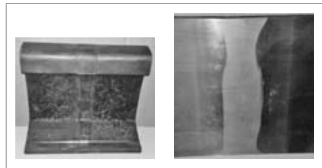
Figure 11 Front view and longitudinal cross section of flash resistance upset welded joint
