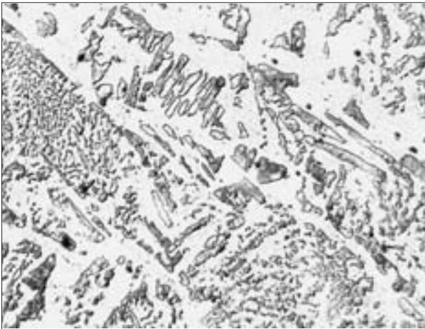
Figure 6 Microstructure of weld metal (Figure 5, location 1)
