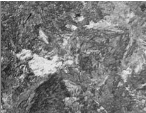
Figure 13 Microstructure of heat affected zone of weld joint from Figure 11.
