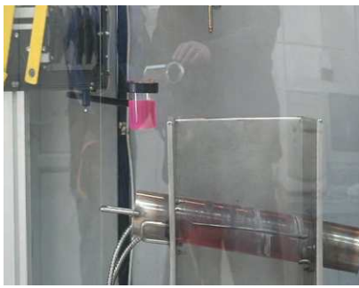
Figure 5. Consecutive images from the film recorded for the fluid HFC Prista, tested at 700°C
