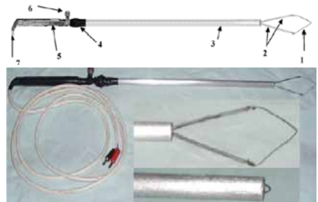
Figure 2: Laparoscopic thermocautery tool (9). 1. Thermal wire; 2. the two movable arms (length, 7 cm) for holding of thermal wire; 3. outer body (metallic tube with an outer diameter 10 mm); 4. rubber valve to prevent gas escape; 5. internal movable part. 6. on/off switch; 7. source of continuous electrical current (12V, 12 A).
