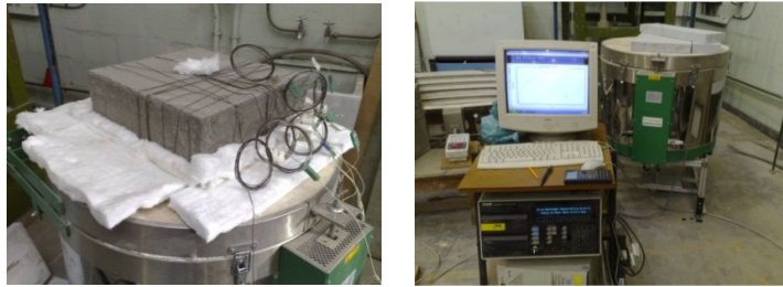
Fig. 13. Typical Set-up for the Small-scale Fire Tests.
