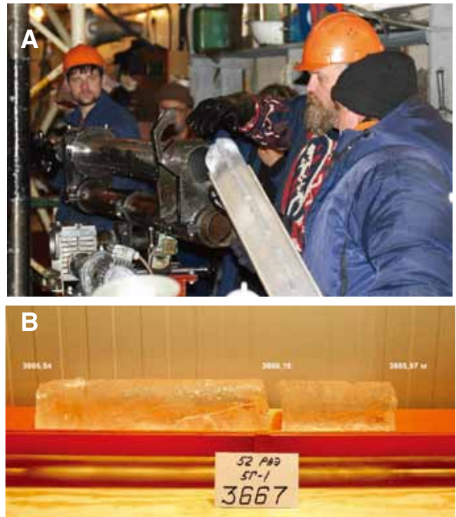
Figure 4. [A] Core recovering from the core barrel (January 2007). [B] Ice core from the deepest layers.
