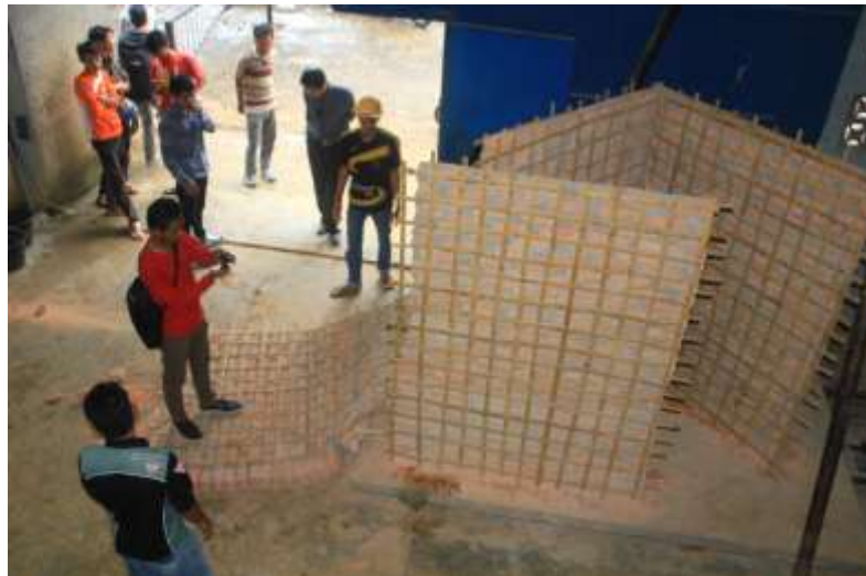
Figure 7. Bamboo wall after shake table testing
