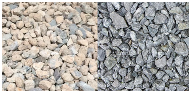
Figure 2: Recycled aggregate concrete (left) and Natural aggregate (right).
