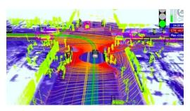
The heart of the system is a laser range finder mounted on the roof of the car. The device generates a 3D map of the environment. The car then combines the laser measurements with the high resolution maps, producing different types of data models that allow the car to drive it while avoiding obstacles and respecting traffic laws.
