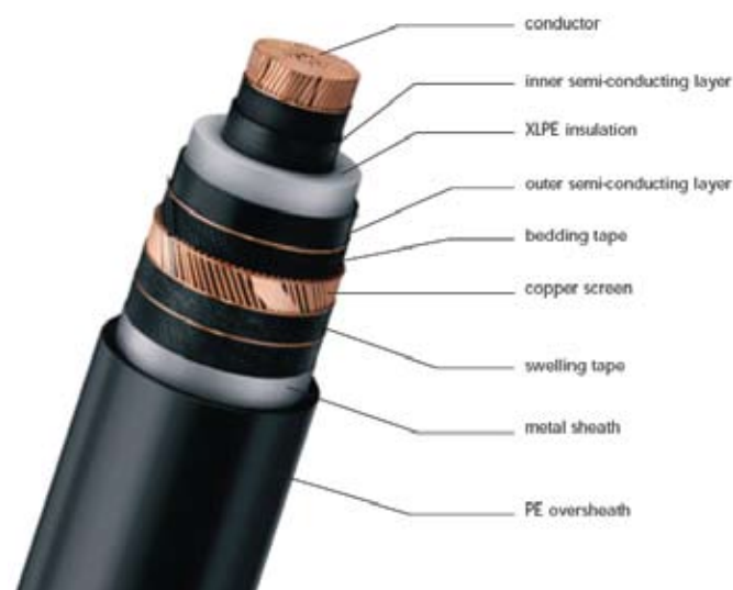
Figure 1. A typical medium voltage cable
