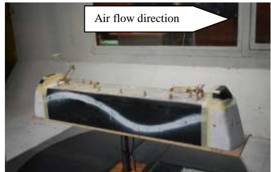
Fig. 16 – Test no. 12 – LE-MA 6000kW with the front pantograph up in the direction of the air flow at the maximum working height and the arms articulation oriented towards the inside of the locomotive and embedded air conditioning
