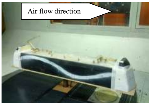
Fig. 17 – Test no. 13 – LE-MA 6000kW with the front pantograph up, in the direction of the air flow at the maximum working height and the arms articulation oriented towards the outside of the locomotive and embedded air conditioning
