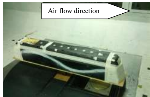
Fig. 18 – Test no. 14 – LE-MA 6000kW with the front pantograph up, in the direction of the air flow at the maximum working height, and the arms articulation oriented towards the outside of the locomotive and streamlined equipment's located on the roof
