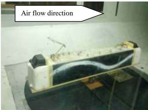
Fig. 11 – Test no. 7 – LE 5100kW with the front pantograph up in the direction of the air flow at the maximum working height and the arms articulation oriented towards the inside of the locomotive and air conditioning located on the box
