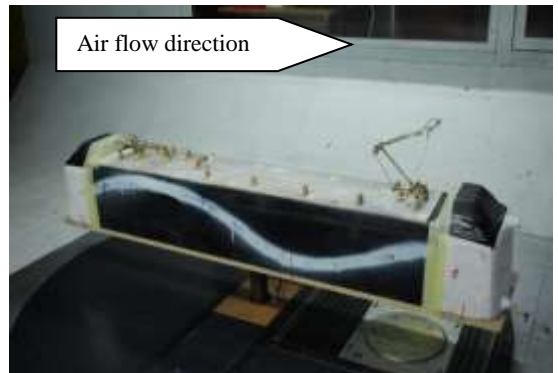
Fig. 12 – Test no. 8 – LE 5100kW with the back pantograph up in the direction of the air flow at the maximum working height and the arms articulation oriented towards the inside of the locomotive and embedded air conditioning
