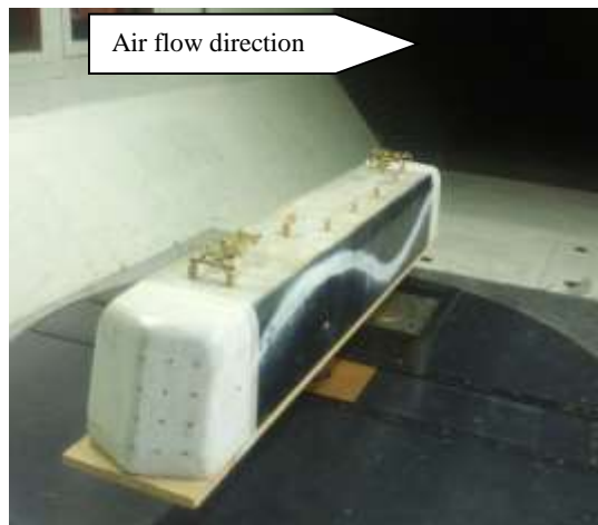
Fig. 21 – Test no. 17 – LE-MA 6000kW with both pantographs lowered and arms articulation oriented towards the inside of the locomotive
