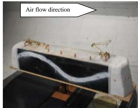
Fig. 20 – Test no. 16 – LE-MA 6000kW with the back pantograph up, in the direction of the air flow at the minimum working height, and the arms articulation oriented towards the inside of the locomotive
