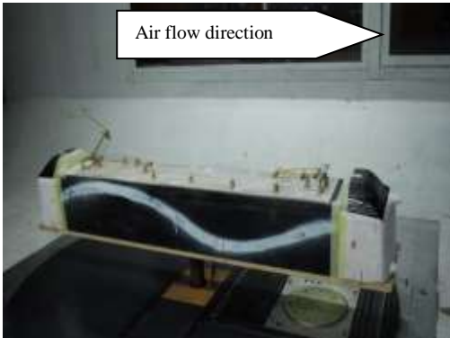
Fig. 13 – Test no. 9 – LE 5100kW with the front pantograph up in the direction of the air flow at the maximum working height and the arms articulation oriented towards the inside of the locomotive and embedded air conditioning
