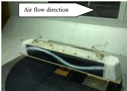
Fig. 15 – Test no. 11 – LE-MA 6000kW with both pantographs raised at maximum working height and articulations of the arms oriented towards the inside of the locomotive
