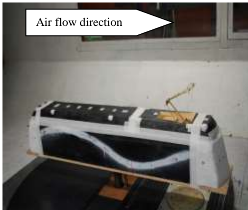
Fig. 19 – Test no. 15 – LE-MA with the back pantograph up, in the direction of the air flow at the maximum working height, and the arms articulation oriented towards the inside of the locomotive and streamlined equipment's located on the roof
