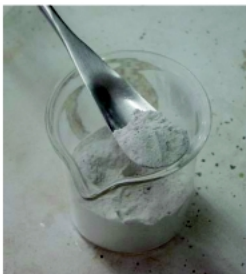
Figure 3. Lime mud after through a sieve No. 100 according to the ASTM standard
