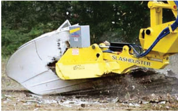
Fig.10. Mechanical cutting of boat hull
