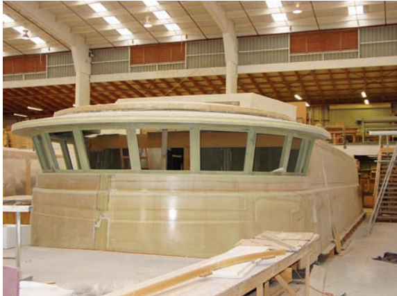
Fig. 3. FRP in superstructure of 33 m HSC yacht
