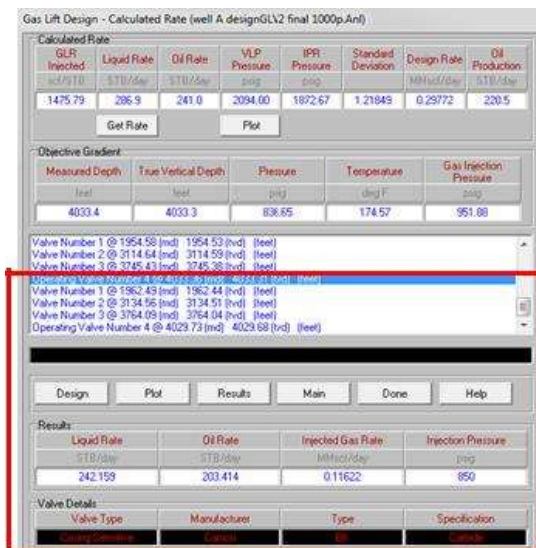
Fig. 5 Optimum Gas Lift Design Prosper will calculate by iteration process to
