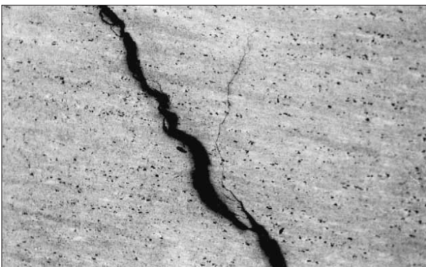
Figure 4 Parallel cracks (OM); magnification 100x.
