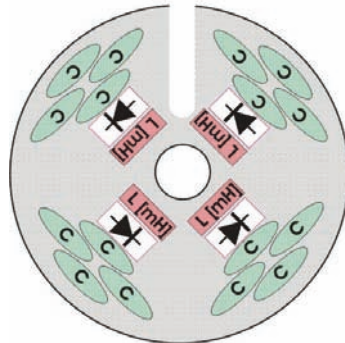
Fig. 4 – One element of the multiresonant circuit within the secondary of the AR70-1000.
