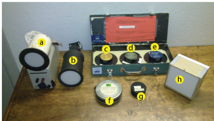
Fig. 2. Some of the low light sources intercalibrated at this workshop: (a) IRF Lauche lamp (SID 101) with power supply, (b) PGI Chernouss-38AM (SID 105), (c) IRF UJO Y275 (SID 5), (d) IRF UJO L1614 (SID 4), (e) IRF UJO 920B (SID 3), (f) FP reference source (SID 1), (g) MPI-2 source (SID 2) and (h) IRF Lycksele lamp (SID 102).
